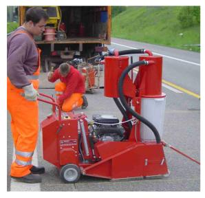
The dry cutting joint tailors Dicorona BS256 has been especially developed to cut induction loops for traffic lights or to cut joints were you can't use any cooling water. In generally the dry cutting process has clear advantages over wet cutting! Some examples:
